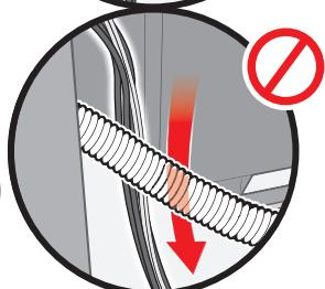
Route wires to the outside of the corrugated gas line.
